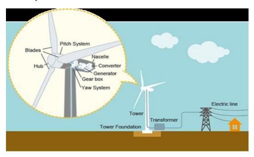
The term rotor refers to the collective assembly of both blades and hub.
